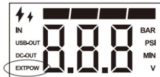
After the EXTPOW icon is on, the following functions are available but the functions cannot be used at the same time.
